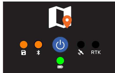
GNSS Module Hardware Error
