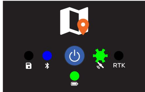
Bluetooth Connected, GNSS Single Fix
