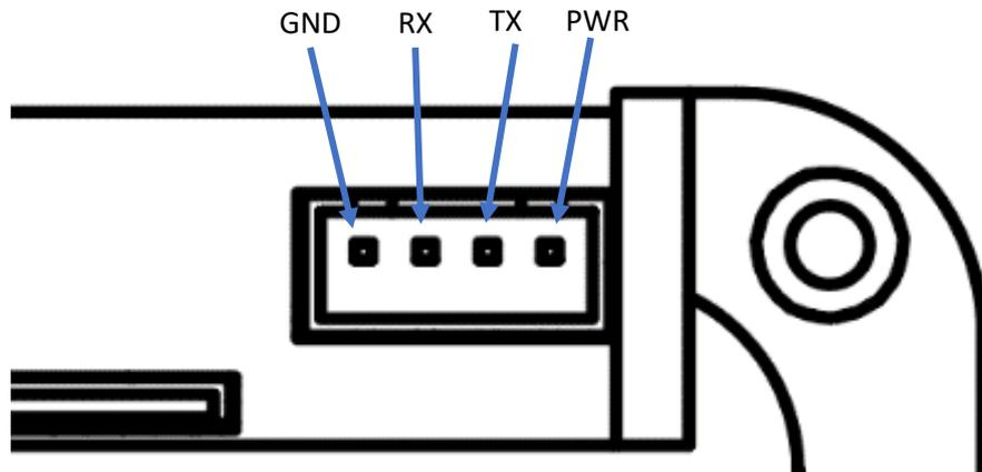
The RX and TX pins are at 3.3V logic level. The PWR pin provides 5V when USB is connected, and the battery voltage (3.5-4.2V) when not. The maximum output current is 1A.
