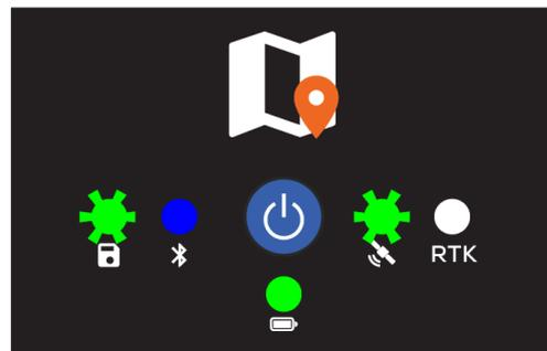
Receiving Radio Weak Signal (Packet Loss)
