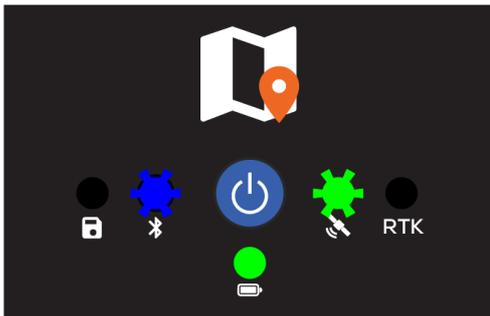
Bluetooth Not Connected GNSS Single Fix
