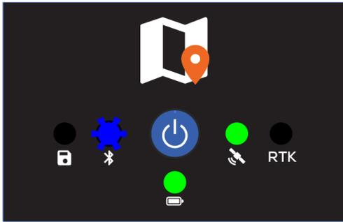
Bluetooth Not Connected, No GNSS Signal
